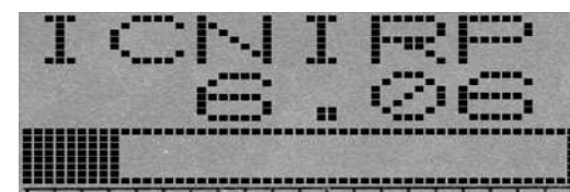
SPECTRAN® displays exposure limits both as percentage as well as a bargraph display.
