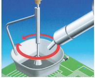
Desoldering IC component with hot air
